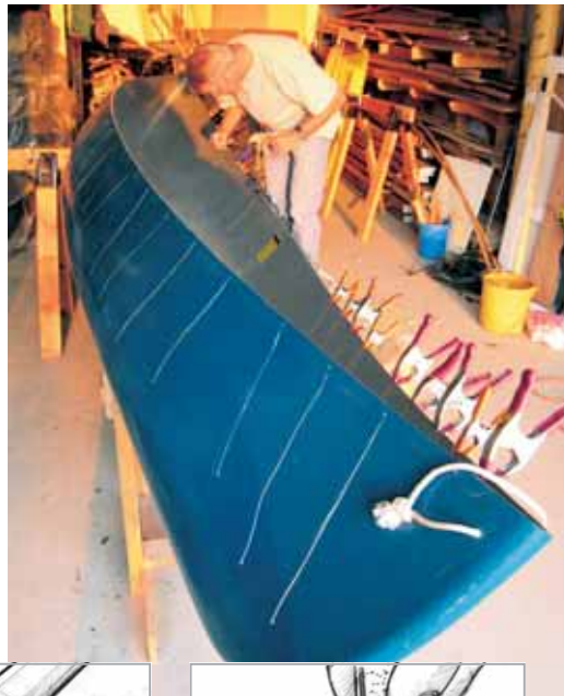
Stan Bradshaw taping cracks on the outside of the canoe with clear tape, readying cracks for G/flex injection.
